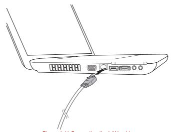
Figure 4-11 Connecting the LAN cable
